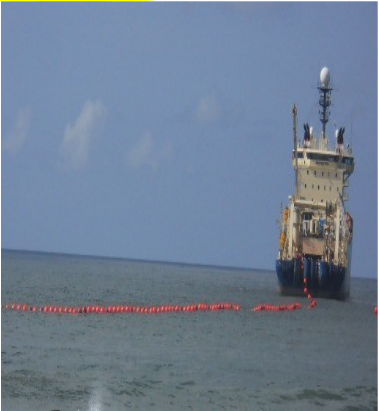
Cable-laying vessel offloading ACE cable on Liberia's coastal waters
